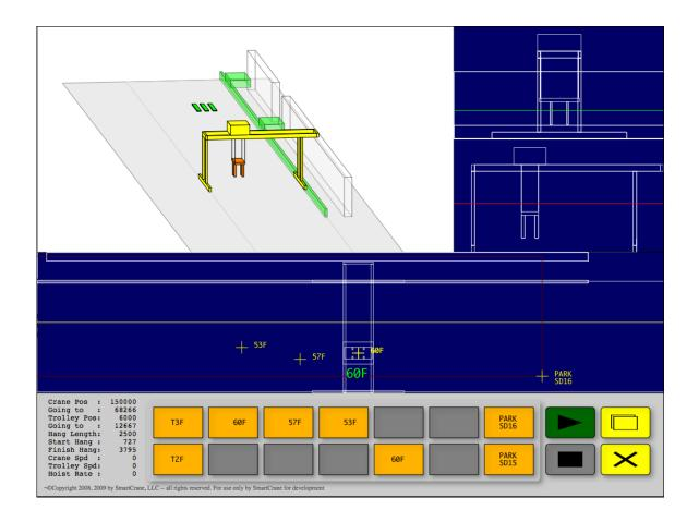
In the upper left are the selectable windows, here showing the 3D display. The operator can change the viewing able and zoom in or out in this window. To the right are two vertical views, showing front and side of the crane. Below is the control view (plan view here) and below that are the control buttons and a real-time data display window.
