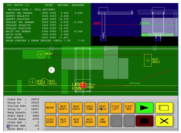
In the upper left as before are selectable windows, here showing inputs from the PLC. An automatic move is just finishing, moving ladle #3 to a destination labeled LADLE FURN. The red line shows the optimal path taken to avoid obstacles in grey-green color.
